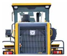
The panorama rear window, high-mounted rear lamps, and reversing alarm equipped ensure good visual field and reversing safety
